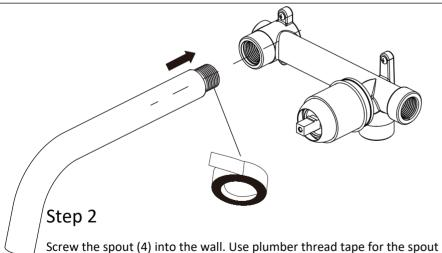
attachment. Screw the spout (4) to the female inlet as shown on the diagram. Ensure the spout is screwed in firmly and the final position has the spout facing straight down.
