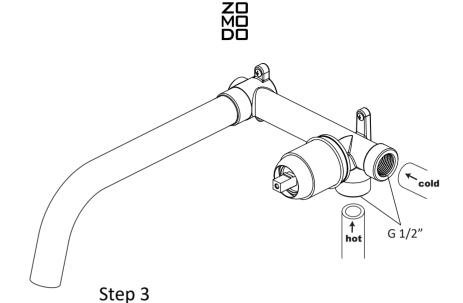
Attach the hot and cold water supply to the other female inlets of the body (9) as shown above.
