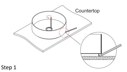
Position the basin in the desired location and with a sharp pencil outline the waste hole. Then scribe outline line around the basin ring (base).
