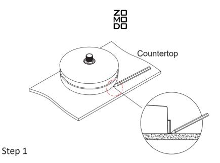
Position the basin/vessel upside-down on the benchtop/counter top in the desired position and draw a pencil line around the basin outer wall.
